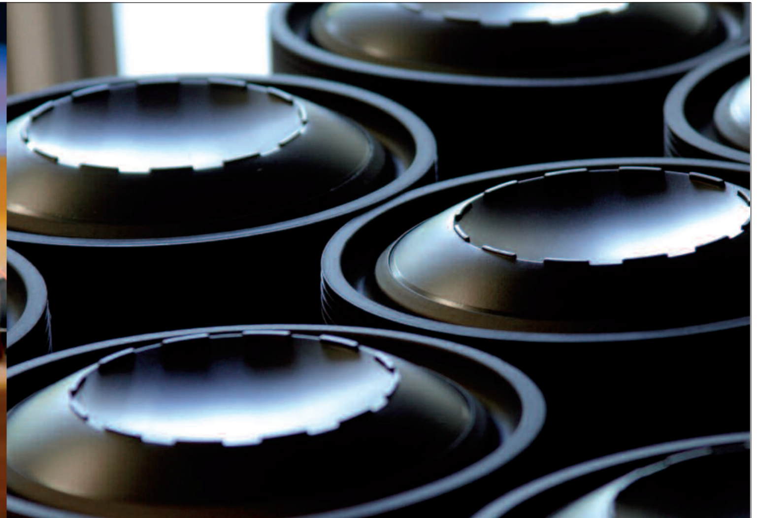
The distinctive Dynaudio cone is manufactured from a single piece of Magnesium-Silicate-Polymer (MSP).
