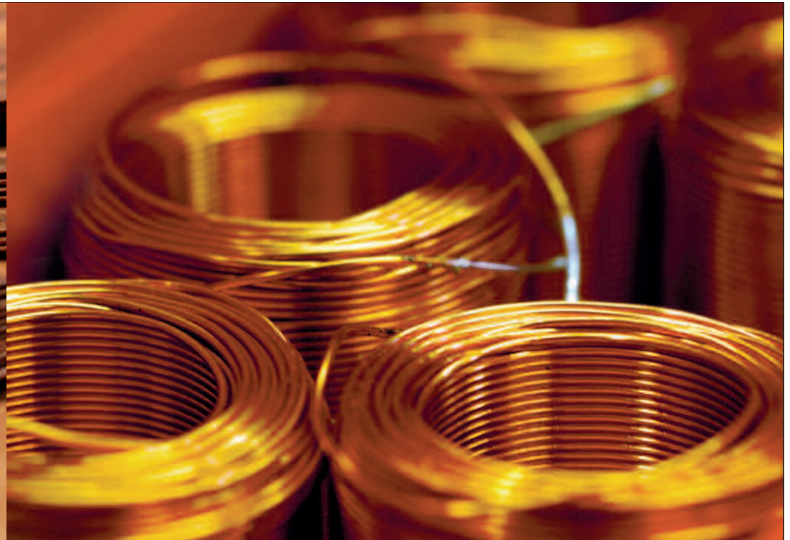
Air-coils wound from the purest grade copper are part of the careful fine-tuning process.
